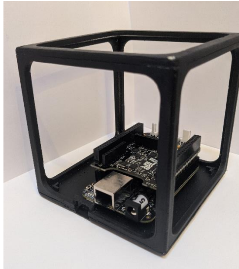
Figure 4.4: The second print of the skeleton casing, housing the Bela board.
